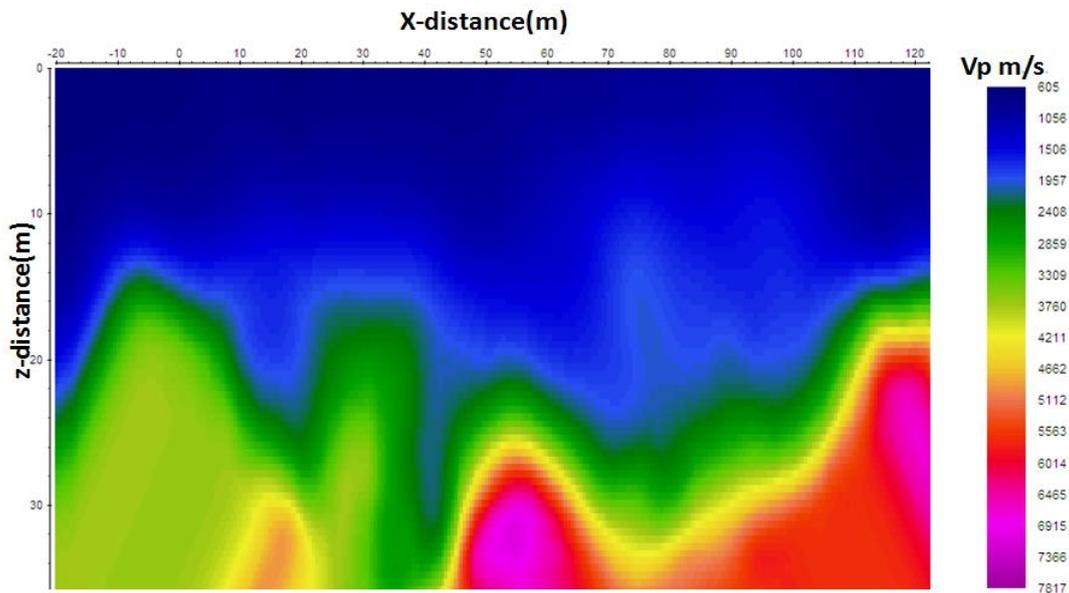
Figure 7: Seismic refraction tomography section along profile C<sub>3</sub>
