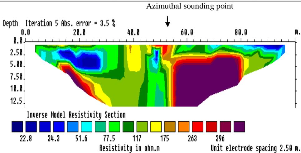
Figure4: Resistivity inverse model along profile C<sub>2</sub>
