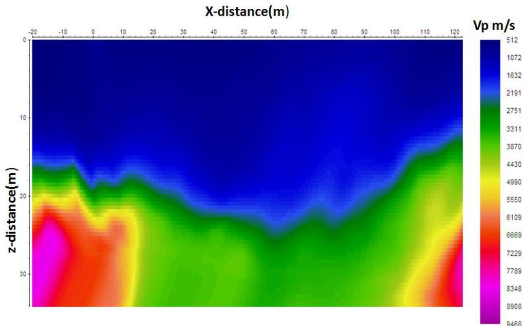
Figure5: Seismic refraction tomography section along profile C<sub>2</sub>
