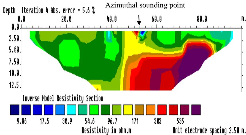
Figure6: Resistivity inverse model along profile C<sub>3</sub>.
