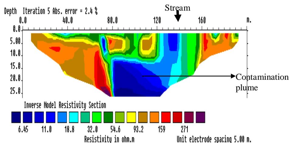
Figure3: Resistivity inverse model along profile C<sub>1</sub>
