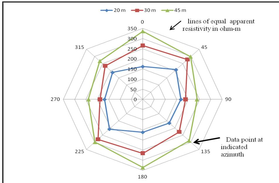
Figure8: Anisotropy polygon at sounding point  $S_1$
