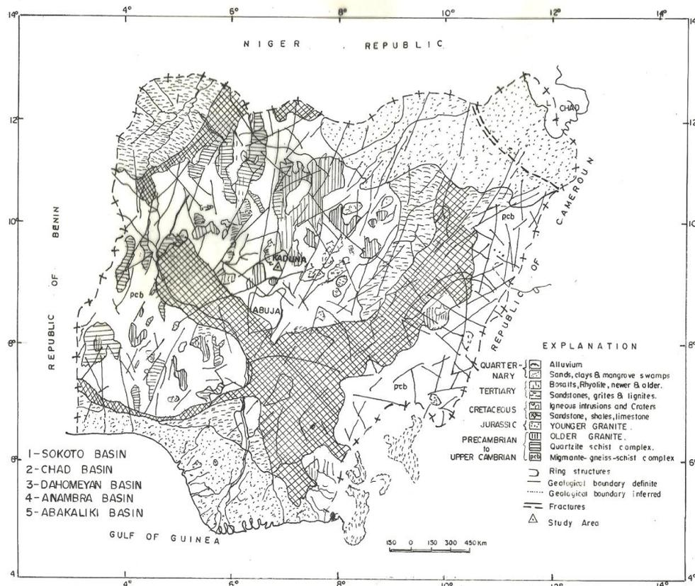
**Figure1: Fracture pattern in Nigeria (Modified after Geological Survey of Nigeria, sheet 2515)**
