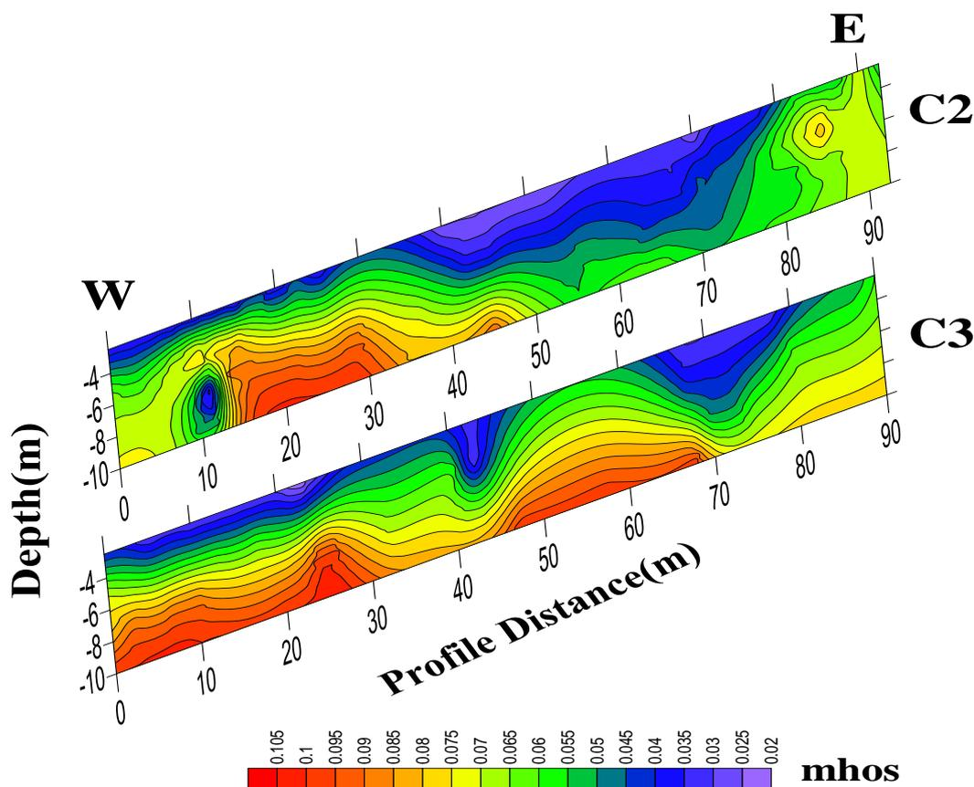
Figure 10: stacked maps of longitudinal conductance along Profile C<sub>2</sub> and C<sub>3</sub>.
