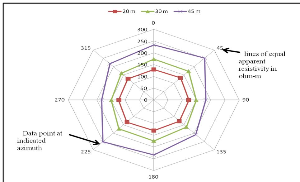
Figure9: Anisotropy polygon at sounding point  $S_2$
